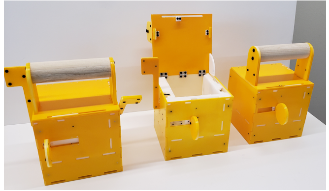
Fig. 2. Completed SMaCK boxes (right to left) slider, slider + lever, slider + lever + dummy lever. Boxes are painted yellow for improved camera visibility.
